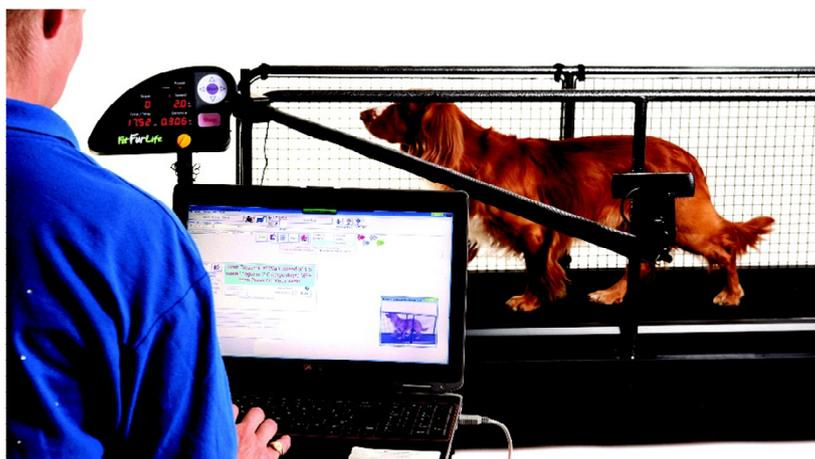
The **GAIT4dog** system, located at Hawksmoor Hydrotherapy (Nuneaton, Warwickshire) is based on the **Fit Fur Life** Professional dog treadmill. It incorporates thousands of tiny sensors under the treadmill belt, which give an unparalleled amount of data which is recorded as a **GLS score**. The system is suitable for most dogs and can be used for dogs from 5 kilos to over 100.
